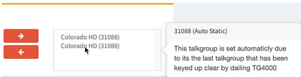
3. In the Pi-Star Active BrandMeister Connections module, which can be enabled via Pi-Star Expert Editor > BrandMeister API, an auto-static talkgroup is listed in the Dynamic TGs list.
